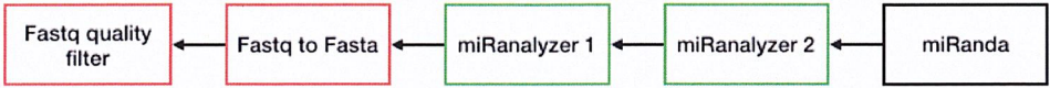
Figure 4.8: Tool queue contain all three queue from different step in the workflow. Red for Pre-processing, green for miRNA Discovery and black for Target Prediction. The head of the queue is on the left side.
