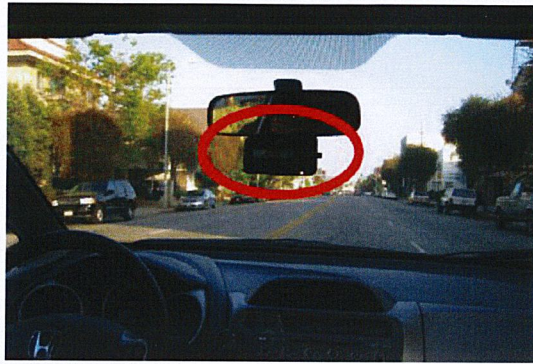
Figure 2.1 SmartLDWS system running on a T-Mobile G1 phone mounted to the windshield of a vehicle
