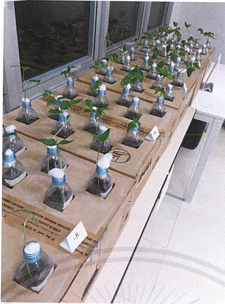
Figure 5.9: Six different trays are also prepared for each type of deficiency of the plant. Each tray can stored up to 12 plants.
