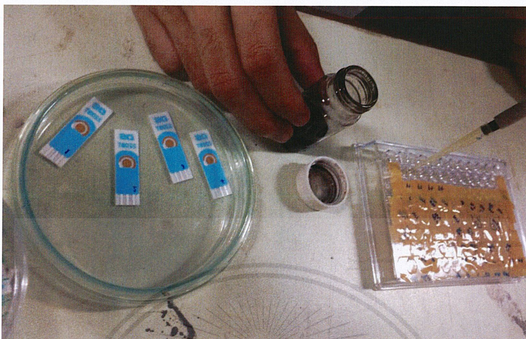
Figure C.5 Prepare for coating polymer on the sensor
