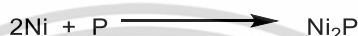
Equation 4 The formation of \text{Ni}_2\text{P} from the reaction between Ni and P.
