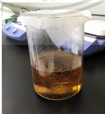
Figure 3.3 Coconut fiber immersed in sodium hydroxide solution.
