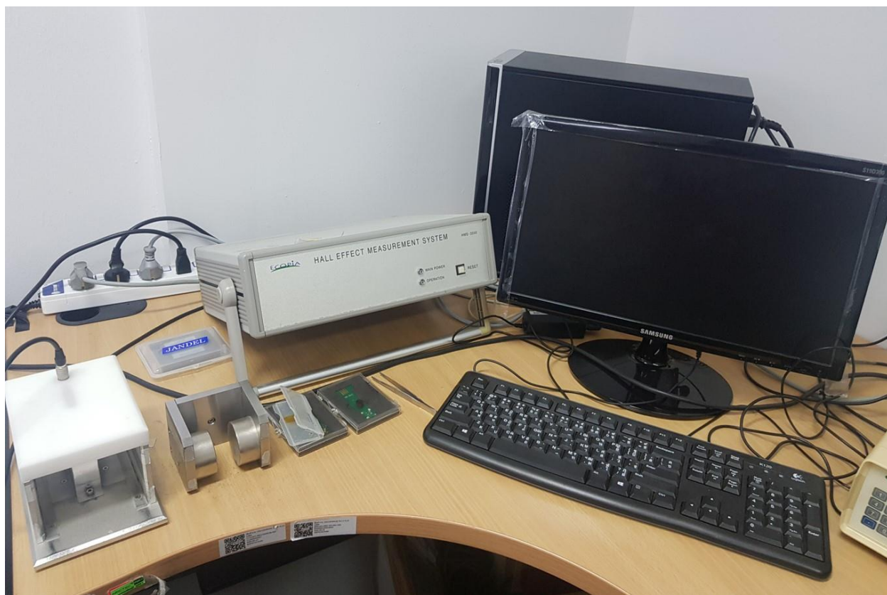
Figure 3.15 Hall effect measurement system (Ecopia, HMS-3000).
