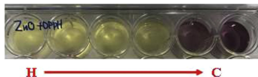
Fig. 3 – Disappearance of 2,2-diphenyl-1-picrylhydrazyl (DPPH*) with respect to the different concentrations of ZnO nanoparticles. C, D, E, F, G, and H represent 0.03125, 0.0625, 0.125, 0.250, 0.500, and 1.000 mg/mL of ZnO nanoparticles, respectively.
