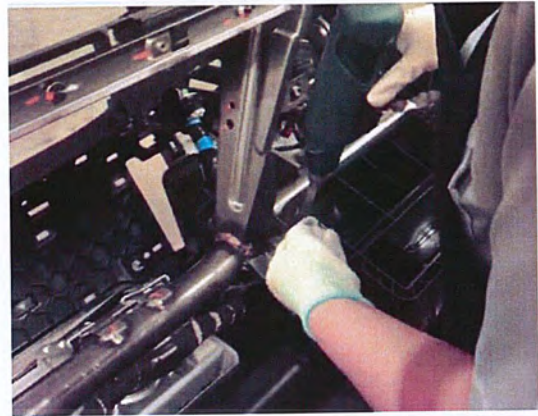
4.Tighten screw at IP skin
