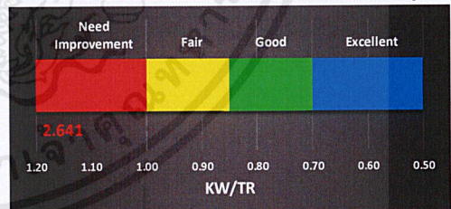
ASHRAE Standard for Chiller Plant Efficiency
