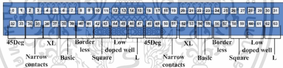
Figure 8. Location of the eight analyzed Hall cells on a tested chip.
