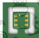
Figure 10 AHT20 top view of printing circuit board. The design of milling slit can minimize heat transfer.
