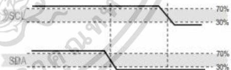
Figure 18 Start Transmit State (S) - When SCL is at high level, SDA is converted from high level to low level. The start state is a special bus state controlled by the main engine, indicating the start of slave machine transit (after Start, BUS is generally considered to be in a busy state).
