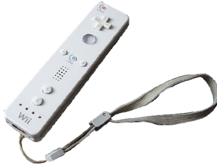
Figure 6: The Wiimote, a device capable of delivering many forms of input and output such as button pressing, position and acceleration of the device, lamp signals, vibration as well as audio output
