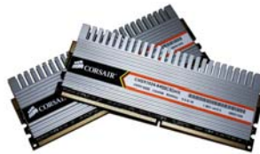
Figure 4: A 2GB DDR2 RAM with integrated heat sinks.
