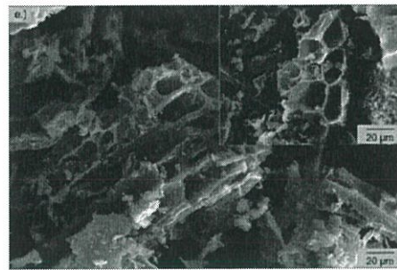
Figure 4. SEM images (300x and 500x) of activated carbons activate with KOH at different temperature (a) 500 °C, (b) 600 °C, (c) 700 °C, (d) 800 °C and (e) 900 °C.
