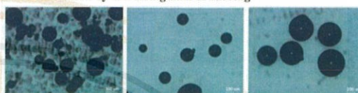
Fig. 3 Optical micrographs of the RF xerogel beads with different stirring times 2 h, 3 h and 5 h
