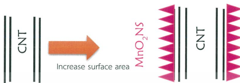
Figure 4.1 Schematic view of \text{MnO}_2\text{-NS} to increase the surface area
