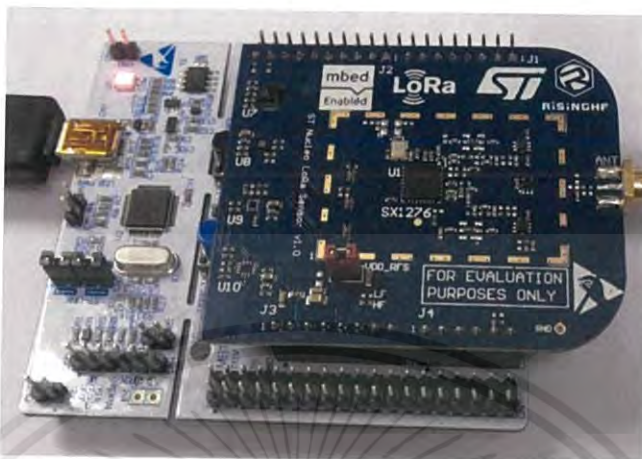
รูป 2.2 LoRa HF band(868/915MHz) RF and sensor expansion board 3
