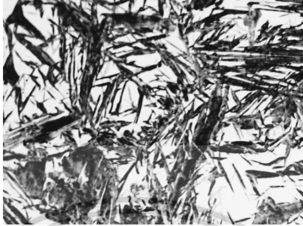
Figure 2.14 Micrograph of martensite microstructure (1220x)
