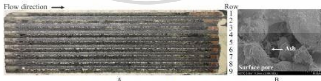
Figures 2. Accumulation of plug ash inside the DPF.
