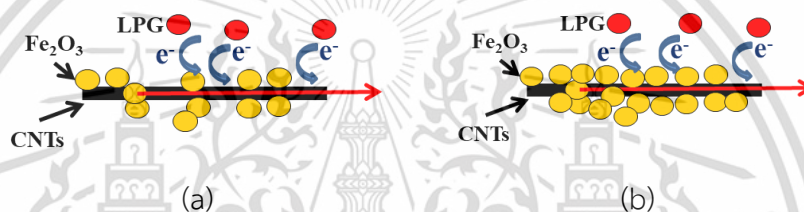
Figure 4.21 Sensing mechanism of (a) CNTs decorated with discrete \text{Fe}_2\text{O}_3 particles and CNTs covered with \text{Fe}_2\text{O}_3 particles.
