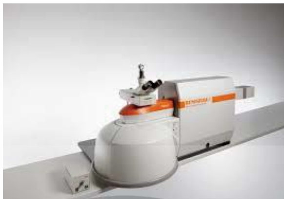
Figure 2.16 Photograph of the Raman spectroscopy (Renishaw inVia Reflex) at Western Digital Thailand [124].
