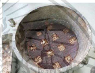
Figure 5. RSS-geogrid installation in the CBR mold.
