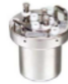
Fig. 2. Test cell for liquid insulation testing "Model DAC-OBE-2".
