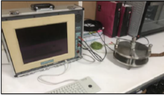
Fig. 3. The PDC measurement for natural ester impregnated pressboard.
