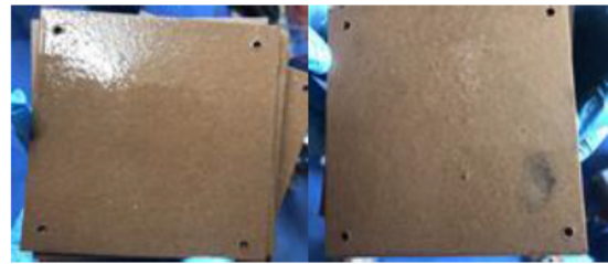
Fig. 1. The examples of the pressboards experienced with the stress voltage of 24 kV for (a) 1 month and (b) 3 months.
