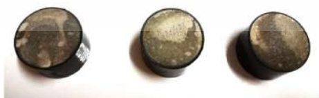
Fig. 9. Moisture ingressive observation on metal oxide block surface.
