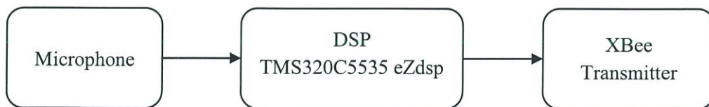
Fig 2: Block diagram of Audio Processing Part
