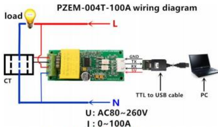
Picture 4.2 PZEM-004T-100A wiring diagram
