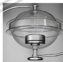
Fig. 6. The temperature controllable chamber a) test chamber dimension, b) designed test chamber, c) test cell with PDIV test electrode and d) test cell with PDC electrode.
