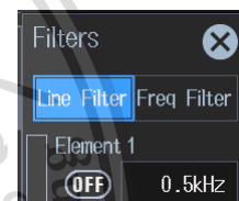
Figure 7. In the Filter menu, line filters and frequency filters for each element can be enabled and adjusted.
