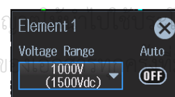
Figure 4. Users can toggle the Auto button to ON for each of the elements.
