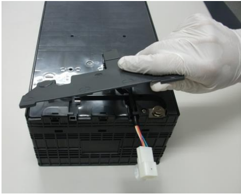
Picture 5-4 Procedure for removal of terminal cover 3
