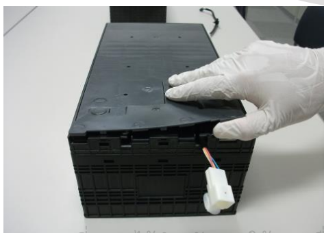
Picture 5-3 Procedure for removal of terminal cover 2
