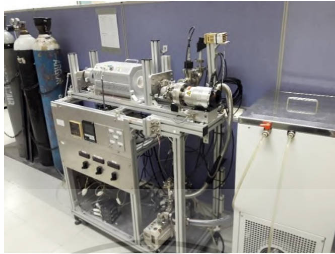
Figure 3.2 Thermal annealing apparatus for annealing of the as-prepared \beta -FeSi 2 samples at different T_{\text{ann}} of 200 °C, 400 °C and 600 °C.
