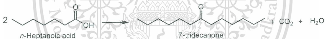
Scheme 4.6 Ketonization of n -heptanoic acid.
