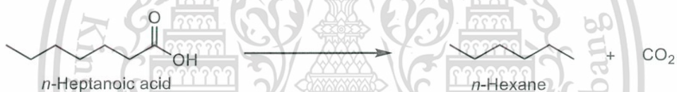
Scheme 4.3 Direct decarboxylation of n -heptanoic acid.
