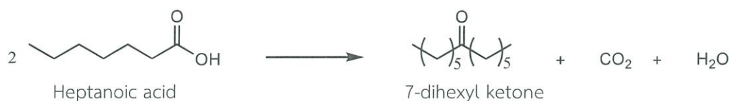
Scheme 2.4 The ketonization of heptanoic acid
