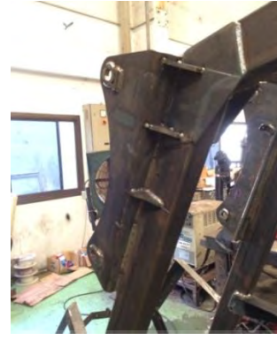
Figure 5.35 Weld loader arm support to frame
