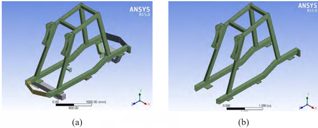
Figure 4.29 Geometry of loader structure, (a) completed FE model, (b) simple FE model
