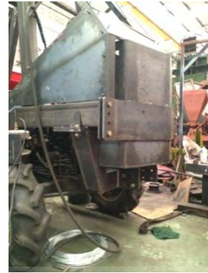
Figure 5.46 Assemble counter weight to loader structure
