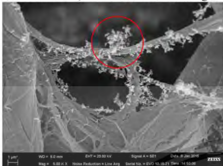
Fig. 14 SEM image of conventional diesel particulate matter in condition of 80% load operation
