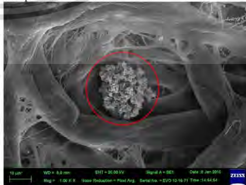
Fig. 13 SEM image of biodiesel blends diesel engine’s PM 10 in the condition of 80% load engine operation.
