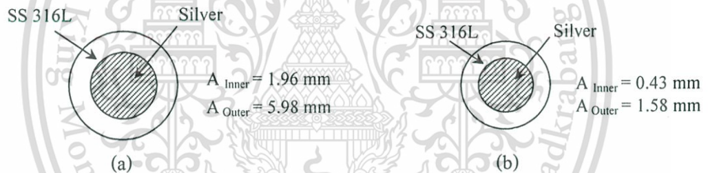
Figure 3.16 Cross-section area of Ag_4968 (a) and Ag_4625 (b).
