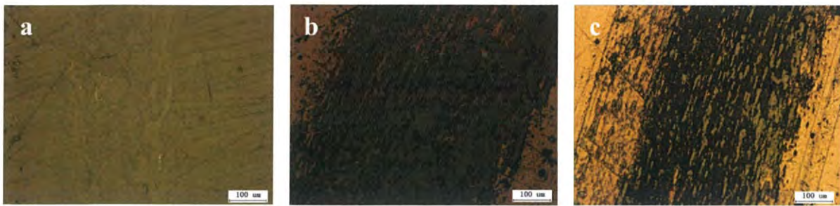
Fig. 6. Photograph form optical microscope of the wear trace of (a) ABS0, (b) ABS125, and (c) ABS175 samples.
