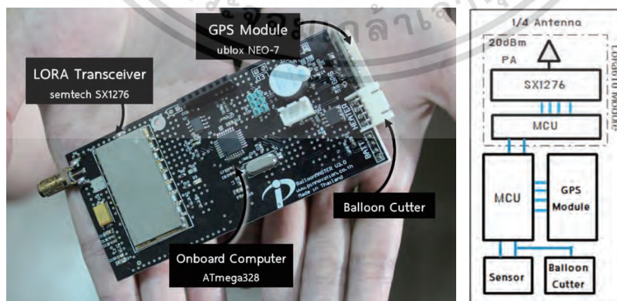
Fig. 8. (Color online) LoRa communication prototype board.
