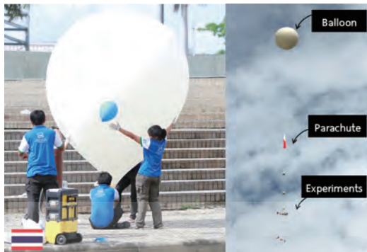
Fig. 11. (Color online) HAB with CubeSat prototype attached.
