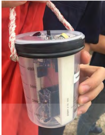
Fig. 3. The designed radiosonde configuration before a test.
