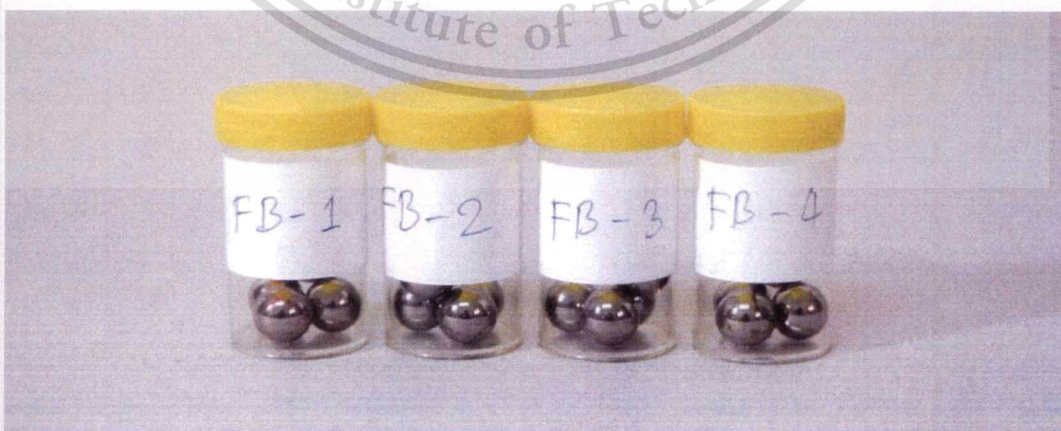
Figure 4-16. Steel balls prepared for Four-ball tribology testing
