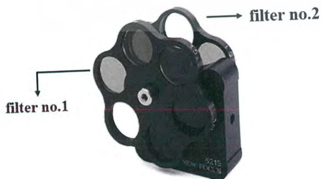
Fig. 3.6 Dual Neutral Density filter wheel for changing the laser power
