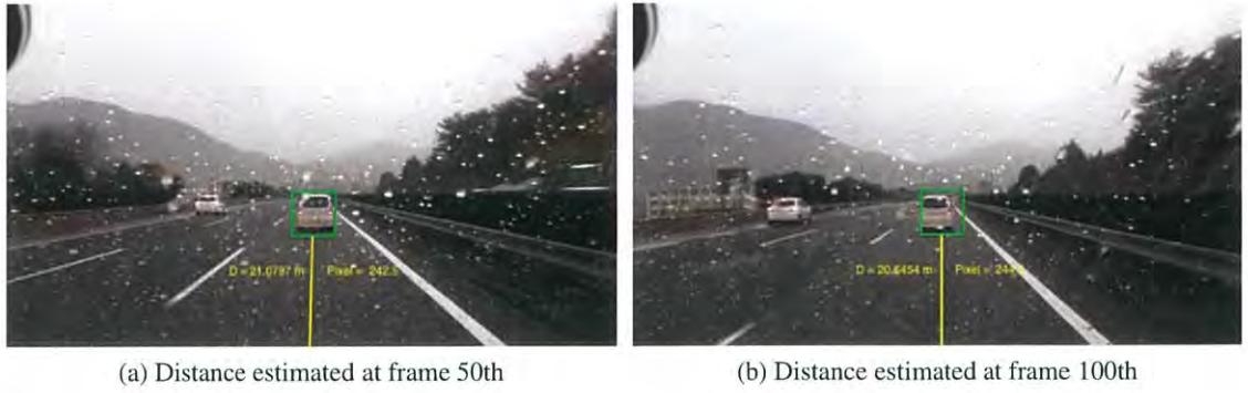
Figure 4.8: Result of distance estimation based on camera-pose-based trigonometric technique
