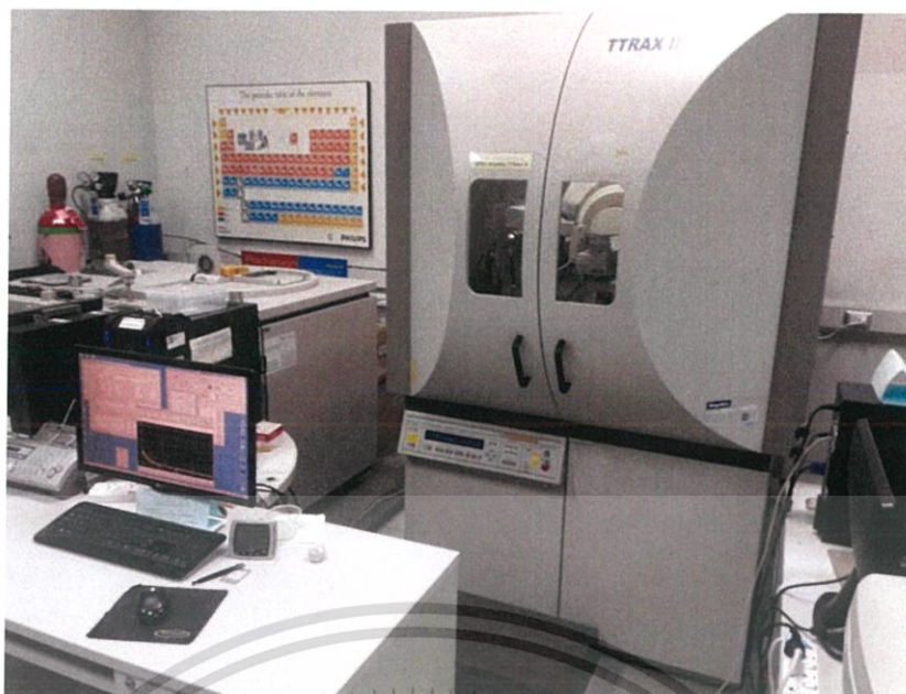
Figure. 3.15 The XRD diffractometer (Rigaku, TTRAX III) at MTEC.
