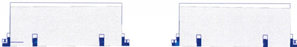
Figure 4.9 The displacement of battery packs of the mounting brackets design during the moment of maximum stress occurrence
