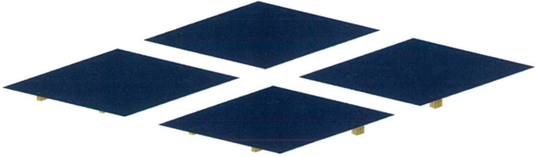
Figure 3.11 Finite element model of battery plate and battery plate tube
