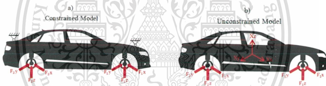
Figure 2.8 a) Constrained model concept, b) Unconstrained model concept
