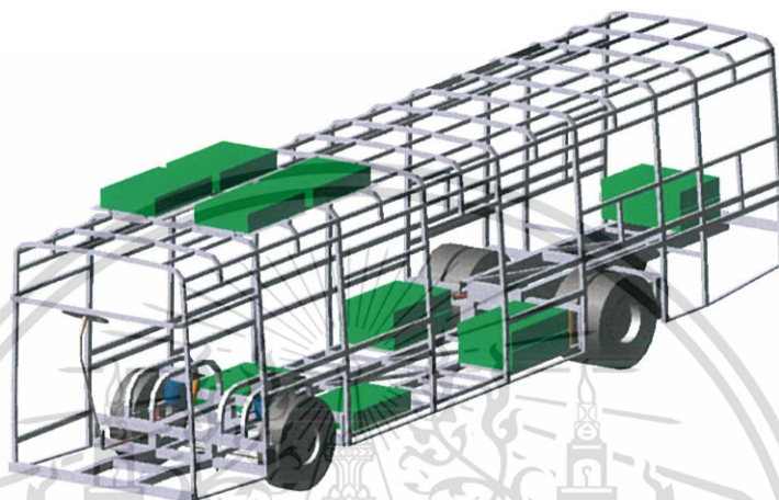
Figure 3.5 Full bus model with battery packs assembled in MSC.ADAMS/Car software
