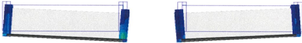
Figure 4.17 The displacement of battery packs of the holder pillar design during the moment of maximum stress occurrence
