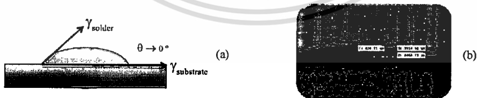
Fig. 4 (a) A schematic diagram for measuring a contact angle of a solder paste on an surface and (b) The measurement of different dimension of a solder paste from its reconstructed image.
