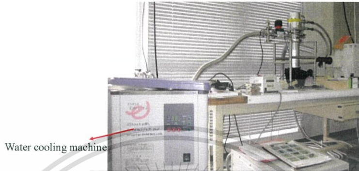
Figure 3.9 Water cooling machine.
