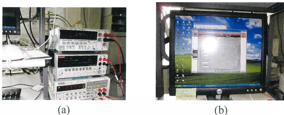
Figure 3.13 (a) The source meter connected with a computer, and (b) program to set the variables of I - V measurement.
