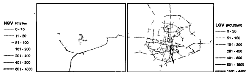
Figure 4.2 (Left) Traffic flow on links in Case I(HGV) (Right) Traffic flow on links in Case I of(LGV)
