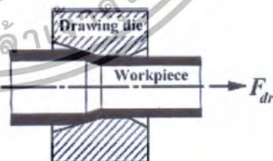
Fig. 1 The principle of tube drawing without a mandrel
