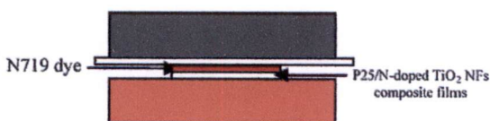
Figure 1 Diagram of dye-sensitized solar cell using P25/N-doped TiO 2 NFs composite film as a working electrode.
