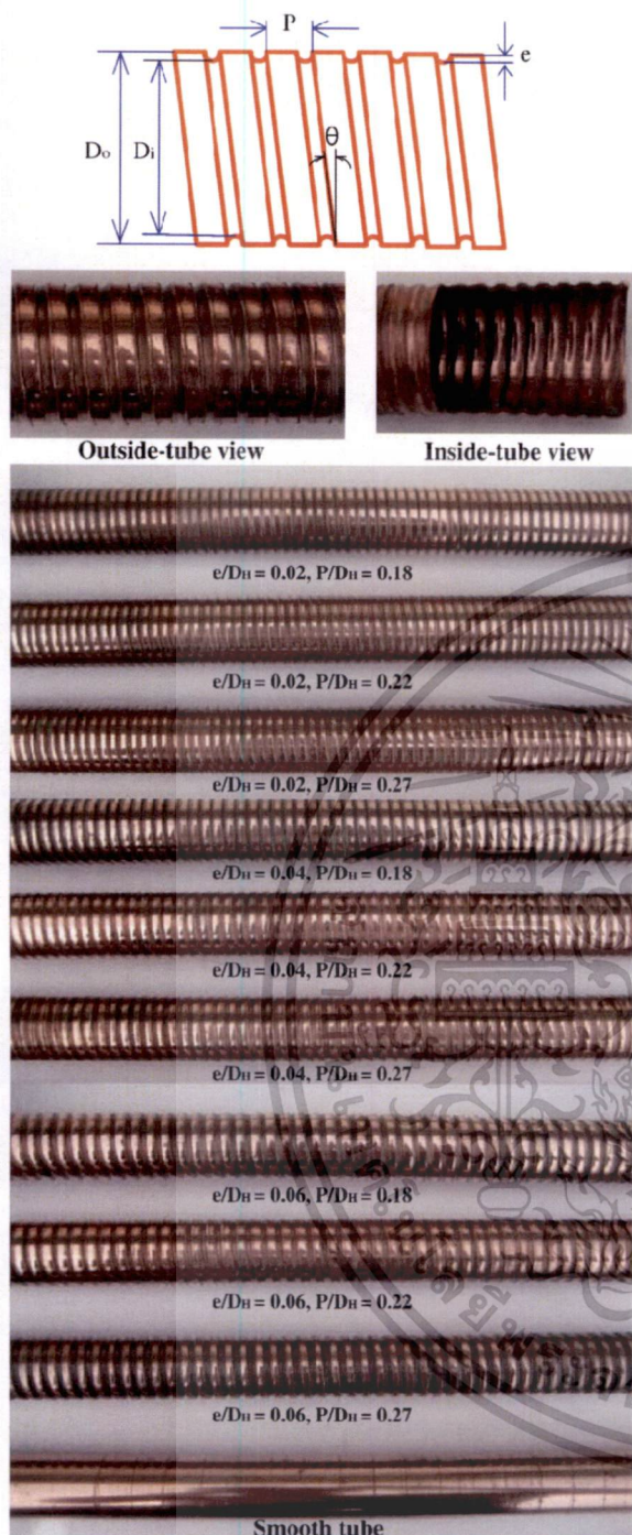
Fig. 2. Photograph of helically-corrugated/smooth tube and definition of geometry.
