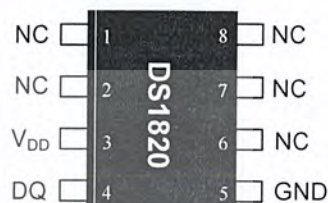
8-pin 150-mil SOIC (DS18S20Z)
