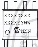
8-Lead SOIC (150 mil)
