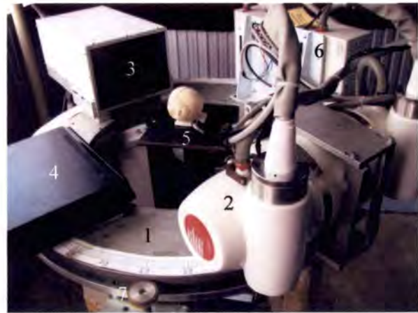
Fig. 2 Small-sized CT system includes 1.) gantry 2.) x-ray tube 3.) x-ray detector 4.) computer for controlling x-ray tube and image acquisition 5.) platform for placing object 6.) cooling system 7.) servo motor for rotating gantry
