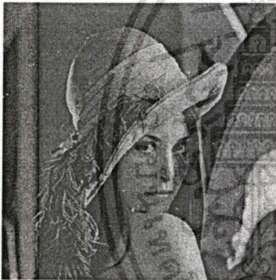
Figure 6: The still image picture at the destination from the source node via sent by multi-hop for the data rate of 110 Mbps. The picture size is 256x256 pixels in gray scale mode.
